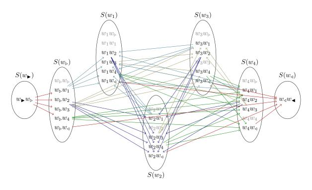
Figure 2. A graph showing the legal transitions between states, when the word-ordering problem is expressed similar to a GA-TSP. Each edge  $\langle w_a, w_b \rangle \rightarrow \langle w_c, w_d \rangle$  has cost  $-\log(P(w_c|w_aw_b))$ . The nodes are grouped into districts (words). Nodes for invalid states are greyed out.
